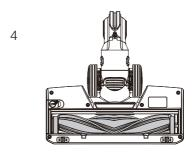
After the cleaning, install the brush roller back.
