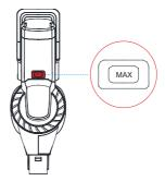
Press the MAX button to go between regular mode (regular power) and MAX mode (max power).
