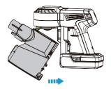
Incline the dustbin, the slot on the dustbin towards the hook on the main body. Push upward until the hook fixed into the slot. A 'click' sound will be heard when it has been successfully accomplished.
