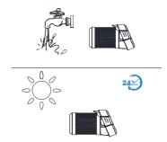
The HEPA can be washed under running water if necessary, and should be dried completely before reinstalling.
